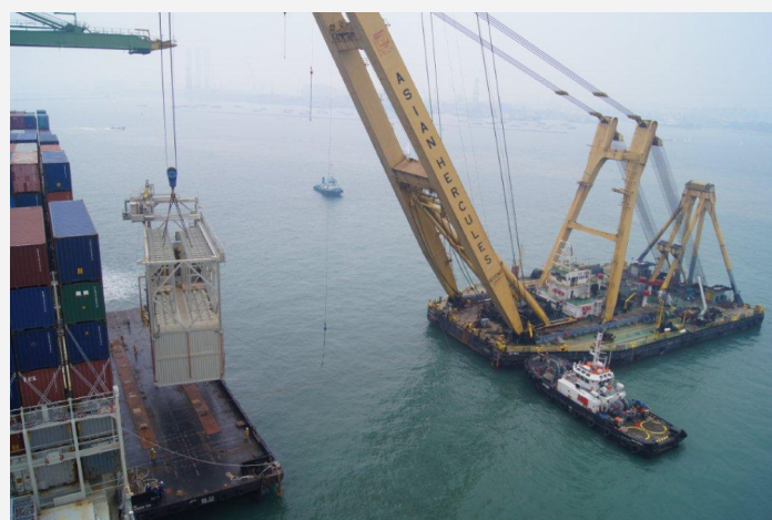
Using a floating crane to discharge a vessel superstructure weighing 450 metric tons from a CMA CGM container ship
