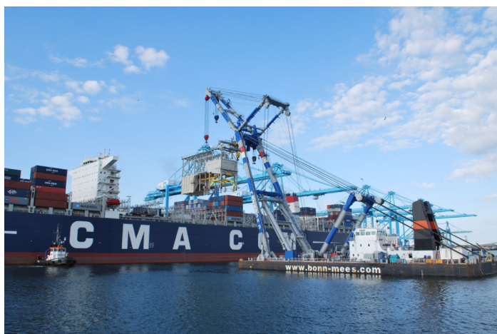
Using a floating crane to load a vessel superstructure weighing 450 metric tons onto a CMA CGM container ship
