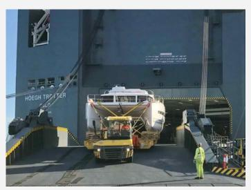
Recently, Höegh Autoliners was chosen to provide the ocean transportation of a 7.12 metre wide catamaran that needed to be shipped from Antwerp to Brisbane. The width of the catamaran was a challenge as it could not be placed on a single 40 foot rolltrailer which has a total width of 2.60 metres.
