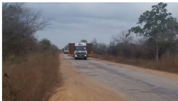
Transport of hydropower plant parts from India to Malawi via Mozambique with cases up to 5.5 m in width
