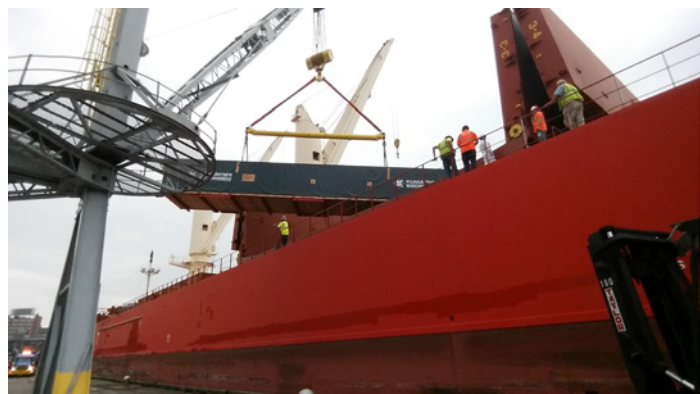
A view from alongside while loading machinery for an airplane manufacturer with cases up to 19.5 x 3.5 x 3 m / 100 tons to the US
