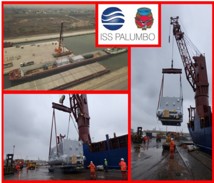
Two steam generators weighing 80 tons each from north Italy to Oman via river barge and subsequent loading onto ocean vessel.
