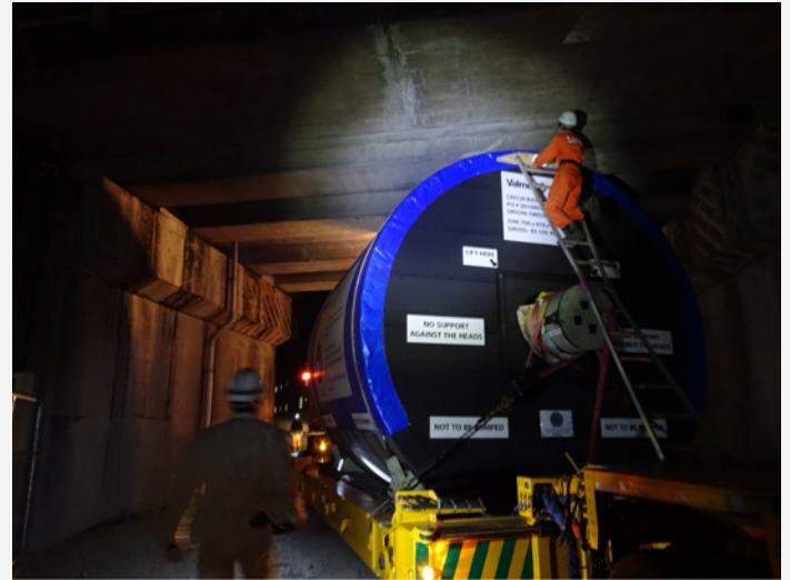
83.1 mt/477 cm high Yankee passing under an 486 cm high Shinkansen (Bullet Train) elevated railway in the middle of the night on 18/Jan, 2018
