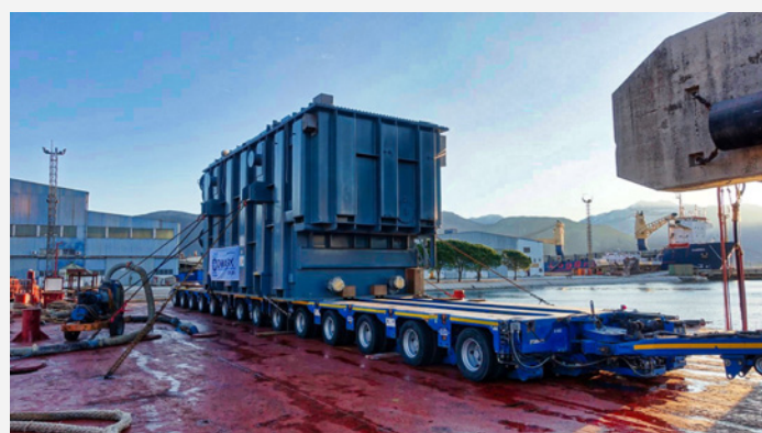
Transformer loaded on a hydraulic trailer onboard a barge
