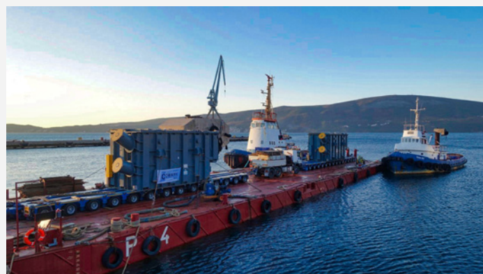
Two of seven 280mt transformers transported by Comark
