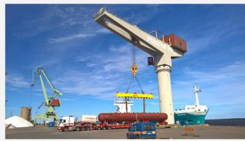
This project cargo was shipped with our feeder vessel m/v Ragna on deck from Hamburg to Rauma. Cargo dimensions: Length: 246cm, Diameter: 285 cm, weight: 161mt. The cargo was discharged in Pori with a 12m lifting boom by the strongest port crane in Finland called "Masa" with a lifting capacity of 200mt
