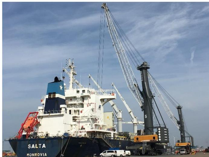
The loading operation passed off without any problems: when the SV Salta weighed anchor, bound for various ports in the Middle East and the Far East, it was at its maximum draft of 13.9 m—full and down. That meant it was carrying 53,000 tonnes of cargo, with a total volume of 64,000 m<sup>3</sup>. The cargo included 30,000 tons of steel slabs, 8,000 tonnes of steel coils, 20,000 m<sup>3</sup> of cast-iron pipes, 6,000 tonnes of pulp in bales and reels and a few smaller shipments of steel.
