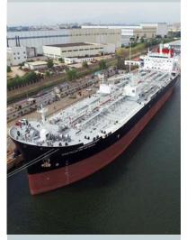
The new ship was built in 2019 and has the last technologies to reduce the emissions of SOx and NOx to the atmosphere by a hybrid "scrubber" in addition to a waste water treatment system certified by the International Maritime Organization (IMO) and the United States Coast Guard (USCG).
